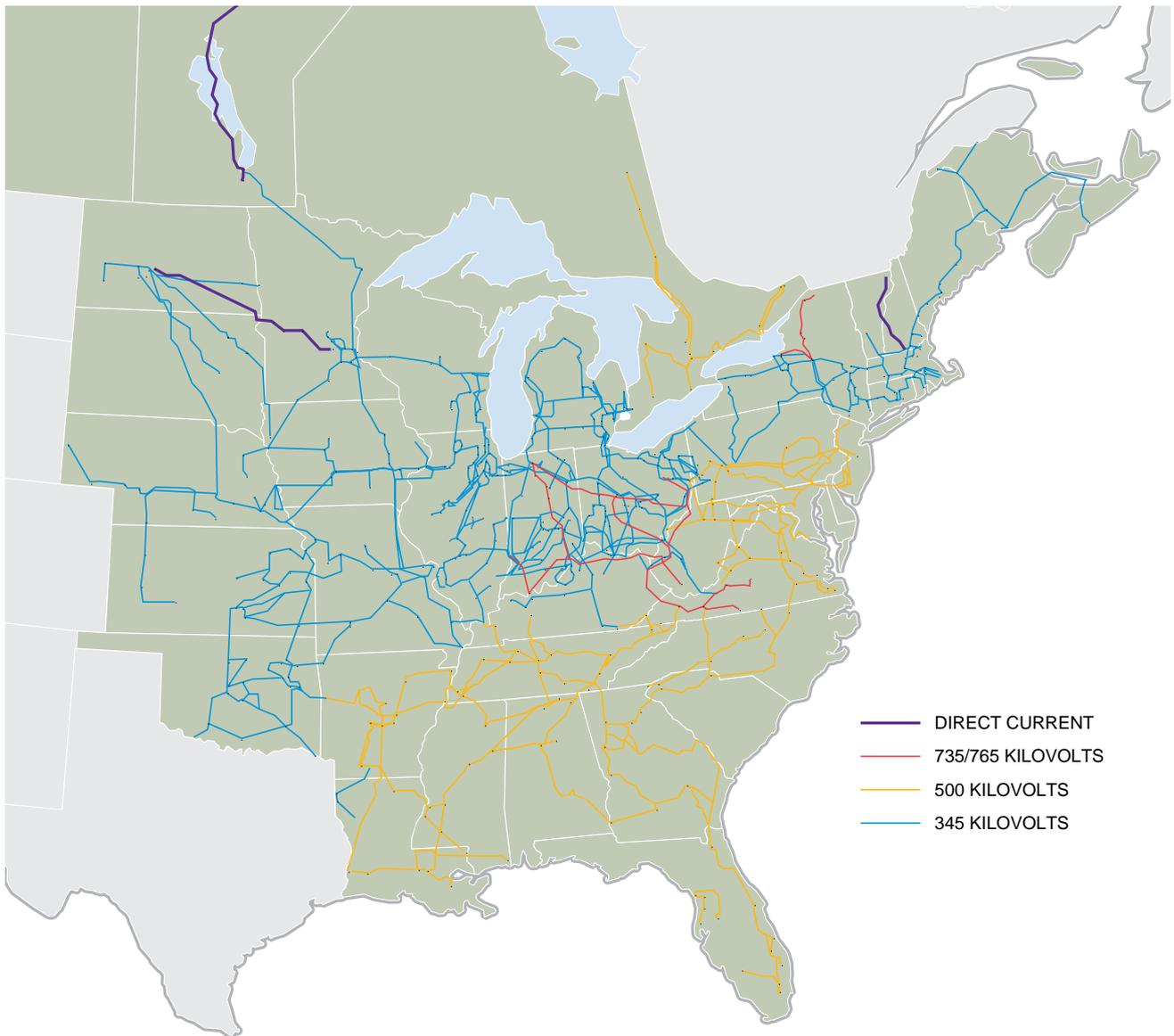
**POWER GRID** ties together most of the U.S. and parts of Canada east of the Mississippi River (*left*). Other networks link the rest of the U.S. and Canada. By adjusting the voltage and
