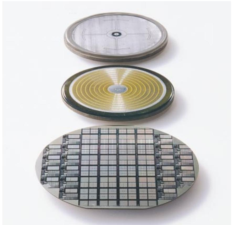
**THREE GENERATIONS** of thyristors show how these devices have increased in complexity and capability. The first-generation silicon-controlled rectifier (*top*) can switch power off only at the beginning of an AC cycle. Gate turn-off devices (*middle*) can switch at any point in the cycle, and MOS-controlled thyristors (*bottom*) switch more quickly while consuming significantly less power.
