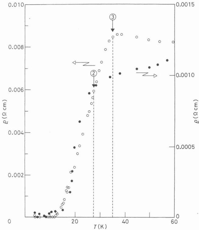
Fig. 2. - Low-temperature resistivity of samples 2 (●) and 3 (○). The onset of the resistivity drop is marked by vertical arrows. Temperature determined with a calibrated silicon diode sensor (DT-500, Lake Shore Cryotronics, Inc.).
