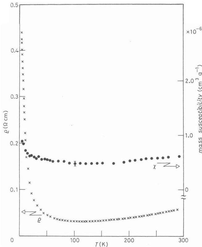
Fig. 1. - Temperature dependence of resistivity ( $\times$ ) and mass susceptibility ( $\bullet$ ) of sample 1.
