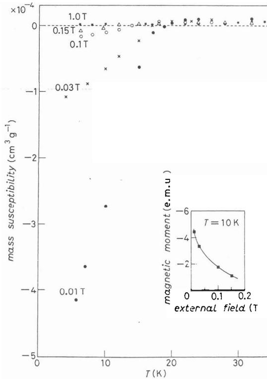
Fig. 4. – Low-temperature susceptibility of sample 2 recorded for different external magnetic fields. The inset shows the field dependence of the magnetic moment at 10 K (sample weight at 0.164 g).
