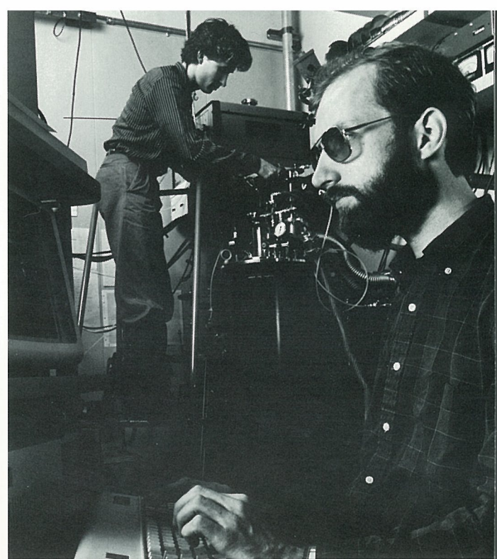
Researchers Stuart Parkin (foreground) and Kevin Roche use a liquid helium cryostat to measure the change in transition temperatures for superconductors in high magnetic fields.
