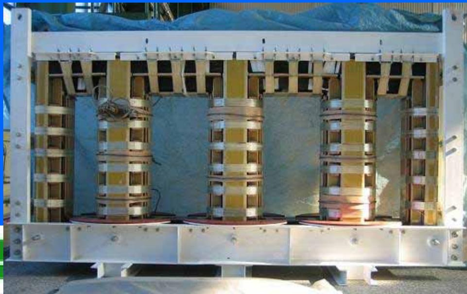
**The iron core was made of amorphous alloy.**
