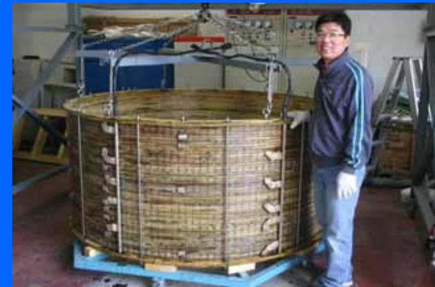
Superconducting coil for FCL
