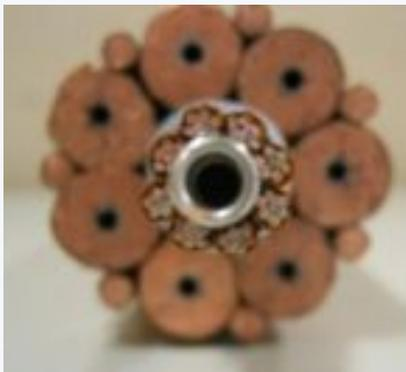
Cable structure using wires
