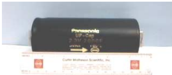
Figure 14-12 Panasonic 2000 F, 2.3 V dc (Six-Inch Ruler Also Shown)
