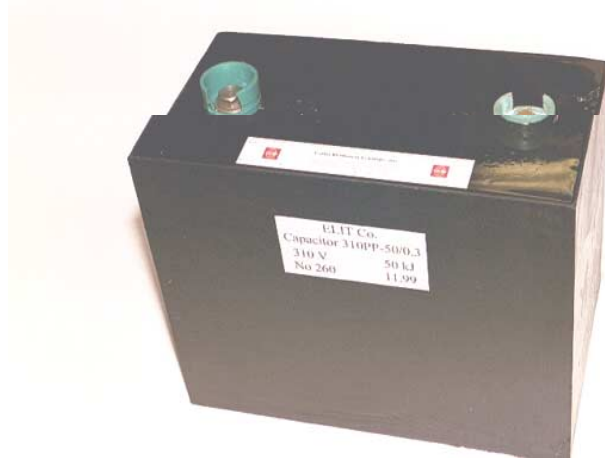
Figure 14-5 Elit Capacitor 0.8 F, 310 V dc , 19 kg (Six-Inch Ruler Also Shown)
