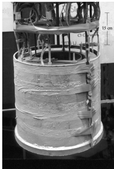
Figure 12-6 1 MJ SMES Coil in a Liquid Helium Vessel (LANL)
