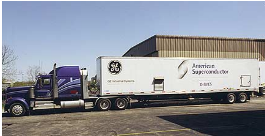
Figure 12-1 A Trailer Mounted D-SMES Unit With 3MW and Up to 16 MVA Capacities (Picture Supplied by American Superconductor)
