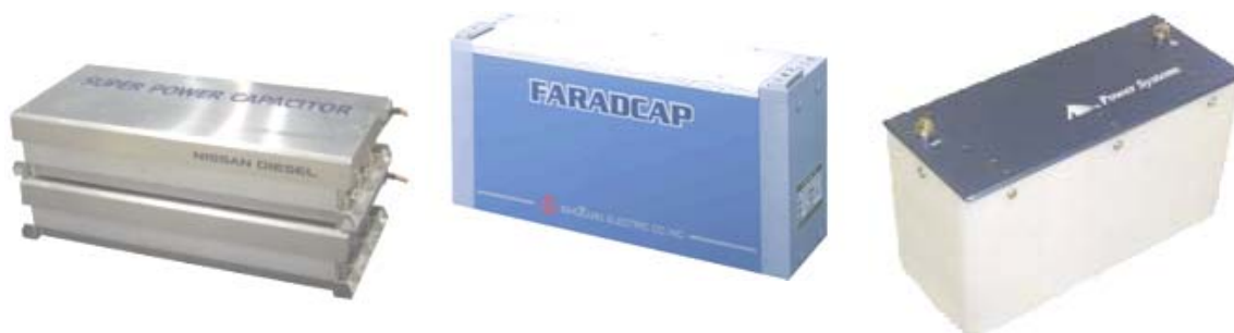
Figure 11 ECaSS commercial capacitors, from left, Nissan Diesel (346Vdc, 35F, 6.3Wh/kg), Shizuki Electric "Faradcap" (FML-2A, 54V, 75F, 30Wh), Power Systems (HO2A, 54V, 65F, 6.5Wh/kg)
