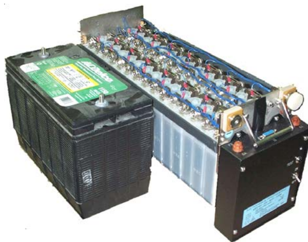
Figure 15 Comparison of physical packages of 12-V, 83A-hour, lead-acid cranking type battery (Delco 1150) and 42-V, 220 kJ, pulse type electrochemical capacitor (ESMA 30EC402)
