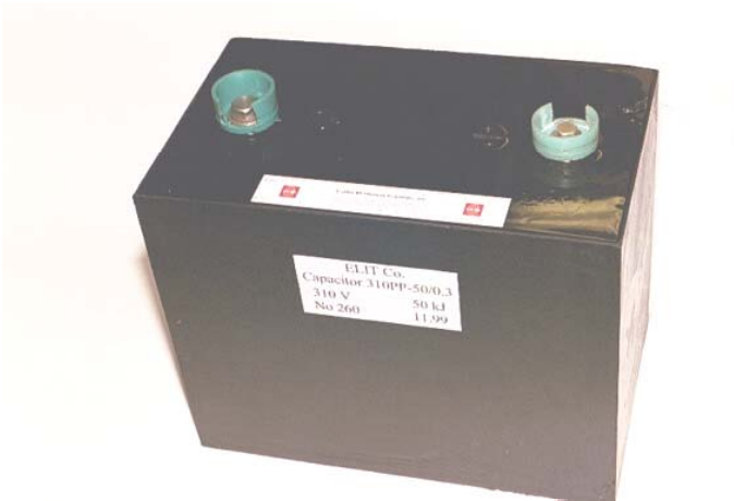
Figure 5 Elit capacitor 0.8 F, 310 V, 19 kg (six inch ruler also shown)
