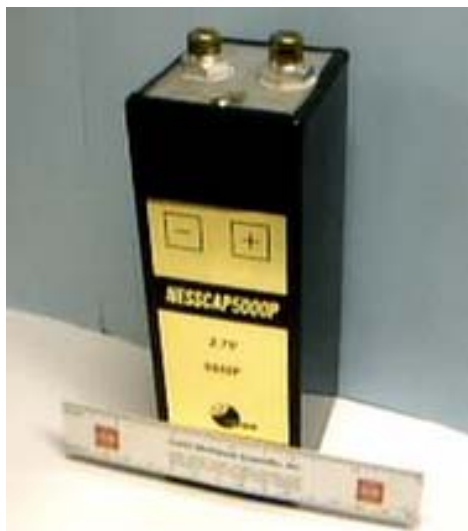
Figure 10 NESS CAP 5000 F, 2.7 V (six inch ruler also shown)
