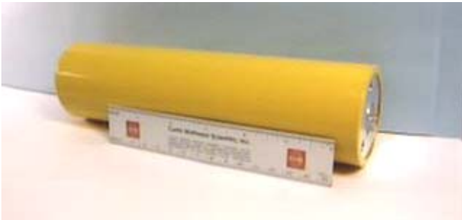
Figure 13 Saft 3200 F, 2.5 V (six-inch ruler also shown)
