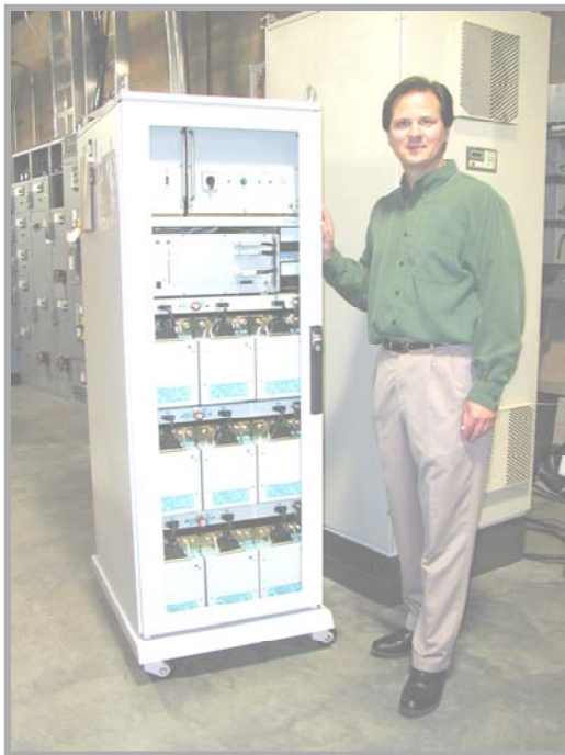
Figure 26 Capacitor System, ~2MJ, 133kW for 15-seconds, energy delivered from dc to dc converters at 600 Vdc, from 9 42Vdc, 220 F Modules operating from 42 to 21 Vdc
