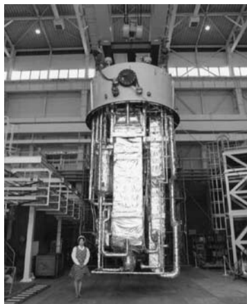
Figure 8 A large liquid helium refrigerator (JAERI)
