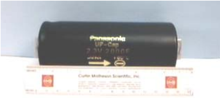
Figure 12 Panasonic 2000 F, 2.3 V (six-inch ruler also shown)
