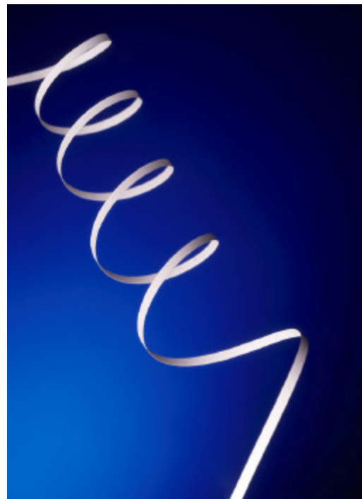
Superconducting tapes are slender and fragile but can carry massive currents.
