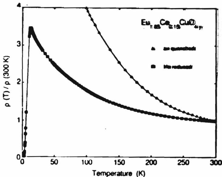
Fig. 3. Normalized electrical resistivity,  $\rho(T)/\rho(300\text{ K})$ , plotted as a function of temperature  $T$  for two  $\text{Eu}_{1.85}\text{Ce}_{0.15}\text{CuO}_{4-y}$  specimens (air-quenched from  $1100^\circ\text{C}$ , triangles; helium-annealed at  $885^\circ\text{C}$ , squares).
