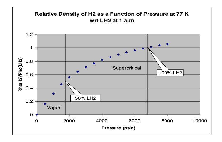
$\rm H_2$  Gas at 77 K and 1850 psia has 50% of the energy content of liquid  $\rm H_2$  and 100% at 6800 psia
