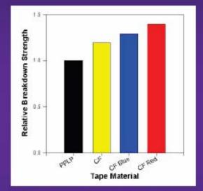
Cryoflex<sup>™</sup> dielectric tape has been improved now can handle 35 kV (200 kV BIL)
