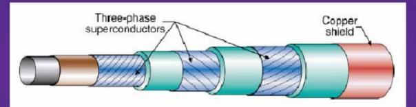
when compared to 3 coaxial phases, tri-axial design promises reduced heat invasion tri-axial design promises reduced need for HTS tape unbalanced impedance no problem for lengths less than 10 km
