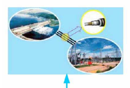
From generator to transformer, typically, 24kV/20-30kA, 20-200m
