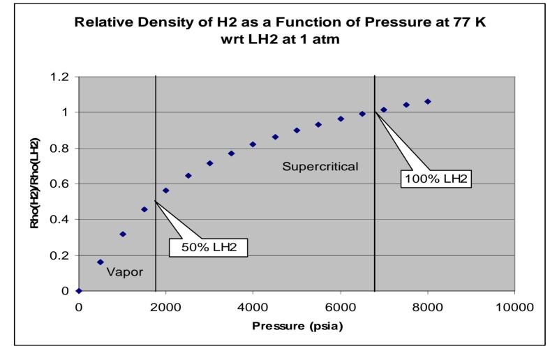
H<sub>2</sub> Gas at 77 K and 1850 psia has 50% of the energy content of liquid H<sub>2</sub> and 100% at 6800 psia !!!
