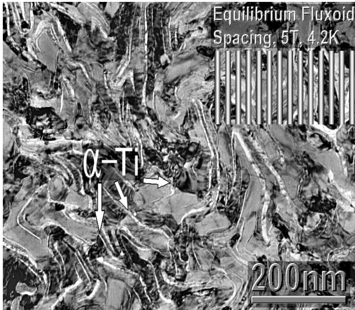
\alpha -Ti ribbons in a Nb-Ti alloy (P. Lee, University of Wisconsin)
