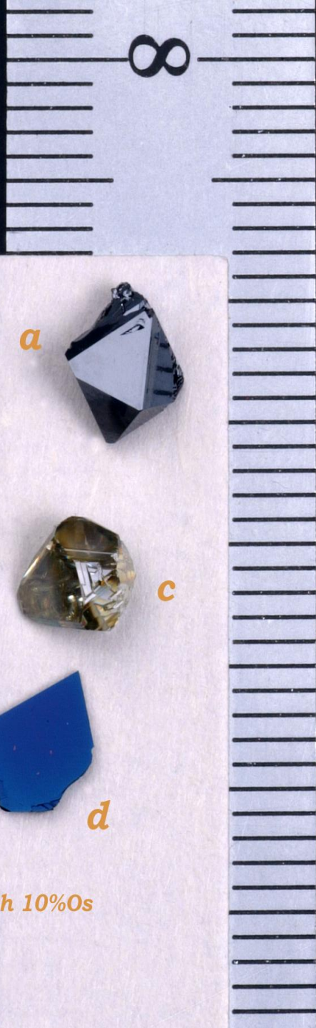
Crystals obtained from chemical transport experiments.
