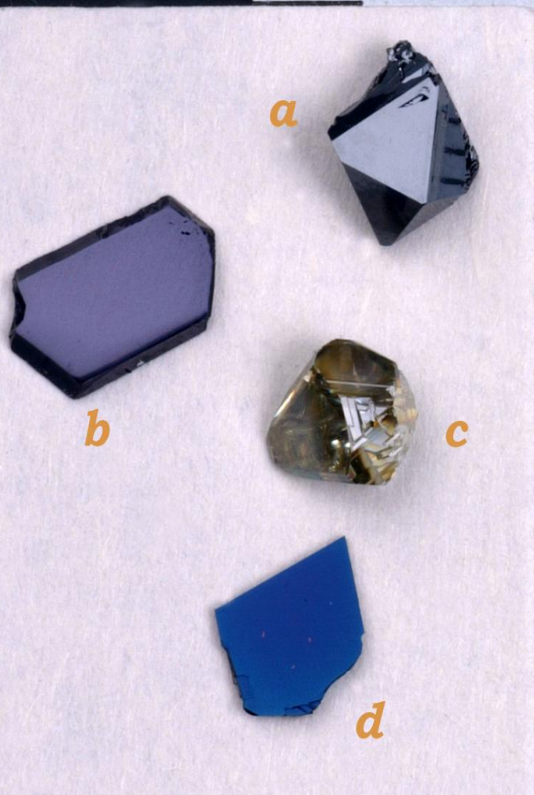
a) Rutil ( \text{TiO}_2 ) with 10%Os b) \text{Cd}_2\text{Re}_2\text{O}_7 c) Anatase ( \text{TiO}_2 ) d) \eta\text{-Mo}_4\text{O}_{11}
