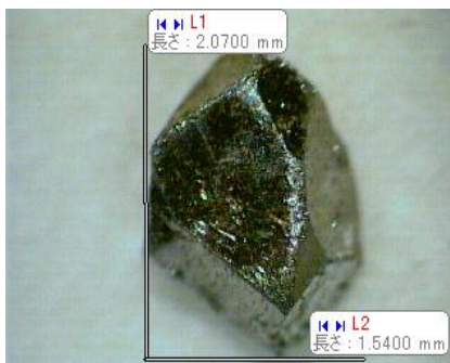
Size of single crystal : 2mm × 1.5mm × 0.5mm
