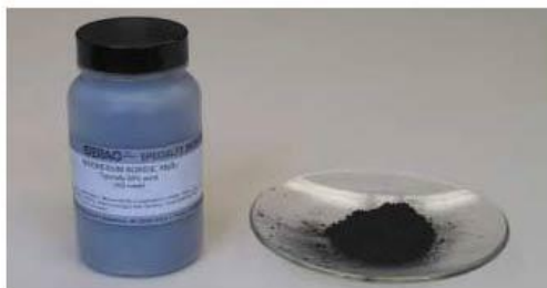
Figure 1 The newly discovered superconductor magnesium boride has been available in large quantities from suppliers of inorganic chemicals for many years, but physicists have finally dubbed the stuff and found that magnesium boride superconducts at an amazing 39 K (ref. 1).
