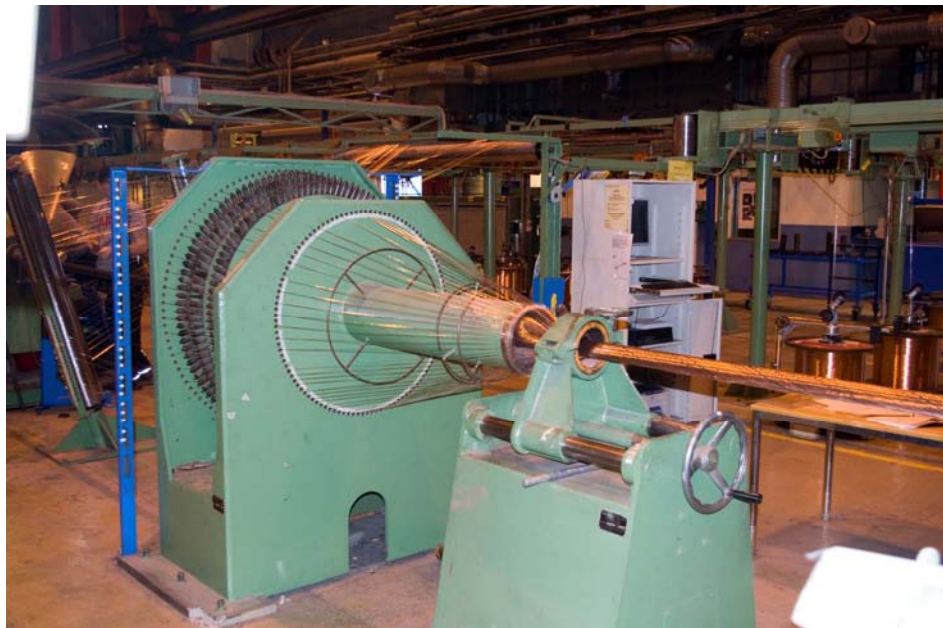
Figure 4-13 Conductor stranding machine
