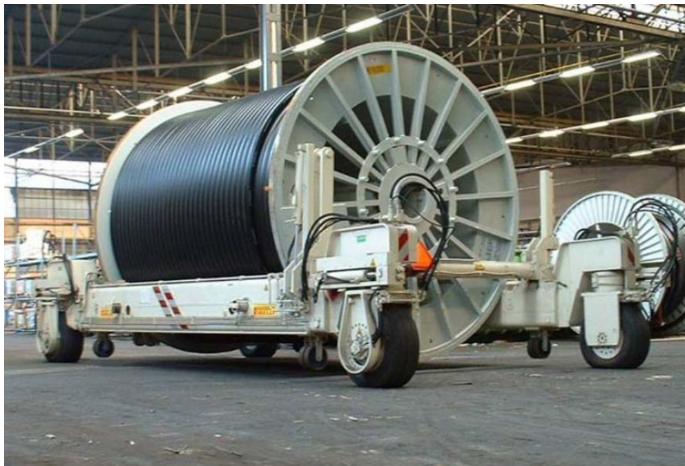
Figure 4-1 Cable transport drum, fully loaded with cable
