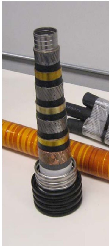
Figure 4-10 A superconducting triplex with nitrogen-impregnated, cold insulation between phases
