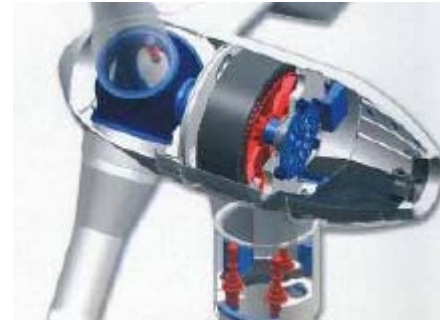
Permanent Magnet No Gearbox
