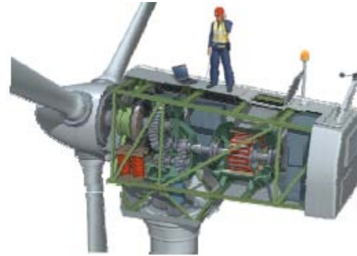
Conventional Turbine Generator
