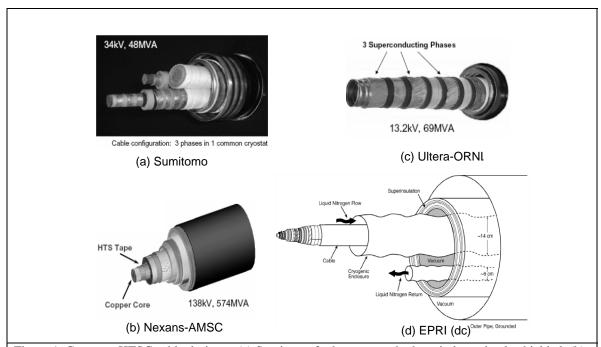
Figure 1 Common HTSC cable designs, (a) Sumitomo 3-phase ac, each phase independently shielded; (b) Nexans-AMSC, high voltage ac coaxial shielded; (c) Ultera-ORNL triaxial, no phase independently shielded; (d) EPRI HTSC dc cable, emphasizing the cryogen flow and enclosure packaging aspects. See each sub-figure to review relative performance parameters.
