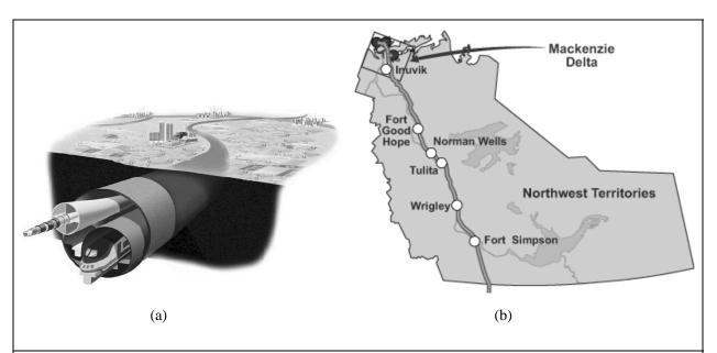
Figure 2 HTSC Cable opportunities for ROW multiple use: (a) Artist's conception of dual use of a tunnel right of way for both high-speed rail and a high capacity HTSC transmission cable, courtesy of Electric Power Research Insitute; (b) The Mackenzie Valley natural gas pipeline route which in principle could support the co-transmission of chemical and electricity power, the latter deploying superconducting cables (see text for explanation)
