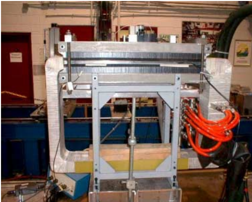
Figure 10.1. Apparatus for magnetic field quality measurements.
