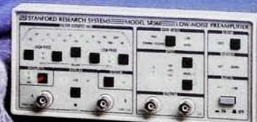
Designed for low noise signal recovery experiments, the SR560 Voltage Preamplifier and SR570 Current Preamplifier are the industry's standards. These general purpose instruments are ideal for amplifying and conditioning very small signals and offer solutions for a variety of photonic and low temperature applications. Both preamplifiers feature a 1 MHz bandwidth, configurable filters, line or battery operation and an RS-232 computer interface.
