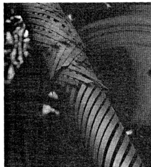
Fig. 29. Finished cable conductor assembly showing first four layers of helically wound tape. The diameter of the conductor is approximately one inch. Photo courtesy of Pirelli Cable USA.
