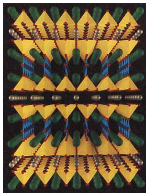
Fig. 3. \text{YBa}_2\text{Cu}_3\text{O}_7 , the green spheres represent barium. For color coding see Figure 1.
