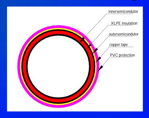
Inner semiconductor shielding layer + Insulation layer +
