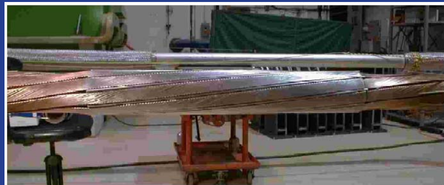
Fig. 6 – Completed splice for the conductor test loop. After soldering, the conductor is wrapped in copper tape to allow clamshell welding of the helium pipe over the splice. The vacuum jacket is made up with telescoping sections over the splice region.
