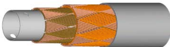
BRAIDED CONDUCTOR (Drive and Current Return)
