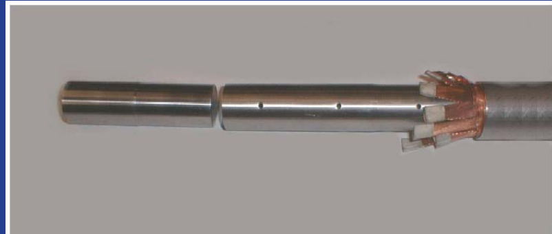
Fig. 4 – End of transmission line conductor. From right to left: Invar pipe jacket, superconducting cables, perforated Invar former, and expanding plug.
