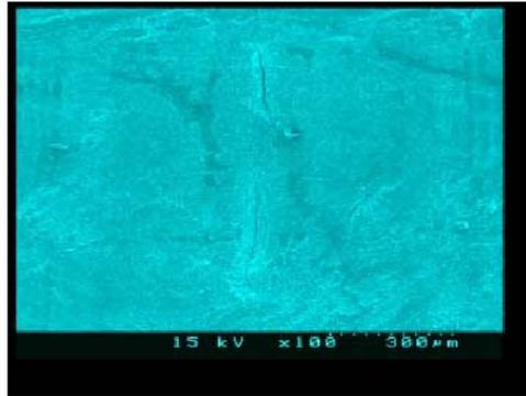
**Fig. 11. Crack in tube 2**
