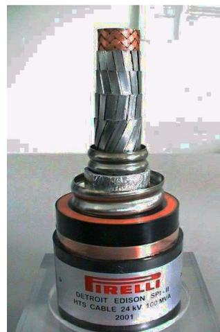
**Figure 2. Cable with Features Displayed**
