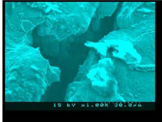
**Fig. 19. Tube 1 detail of crack on inner surface**
