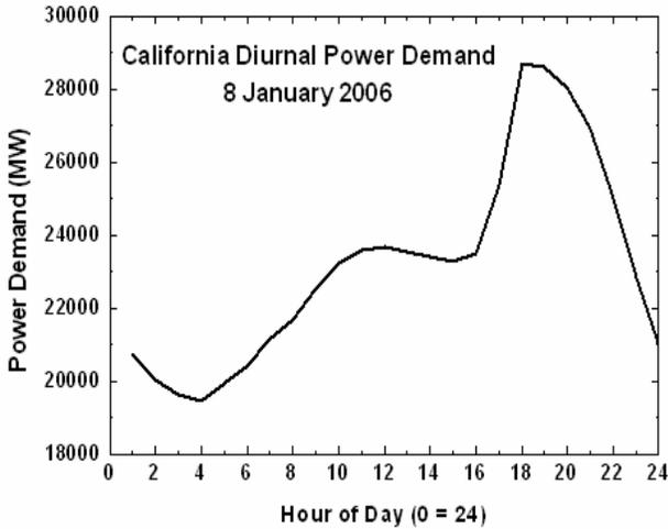
Fig. 4. Actual diurnal load on a typical midwinter Sunday throughout the state of California from 01:00 hours to 24:00 hours [21]. Note the late afternoon “lights on” surge typical of that time of year.
